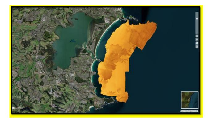
Multibeam backscatter image of the Shellharbour Tharawal marine survey collected by the NSW government (Department of Planning and Environment – DPE) during the period 25 May – 30 November 2017 onboard the RV Bombora using DPE's R2Sonic 2022 multibeam sonar. Light colours indicate relatively softer substrate, while darker colours indicate harder substrate.
